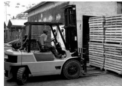
Loading balsa boards into the kiln.
