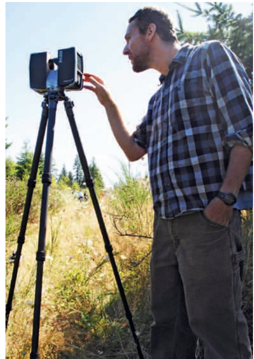
Jeremy Frank, OSU graduate student, inspects a new LIDAR laser scanner that maps forested land to calculate how much carbon is stored there.
