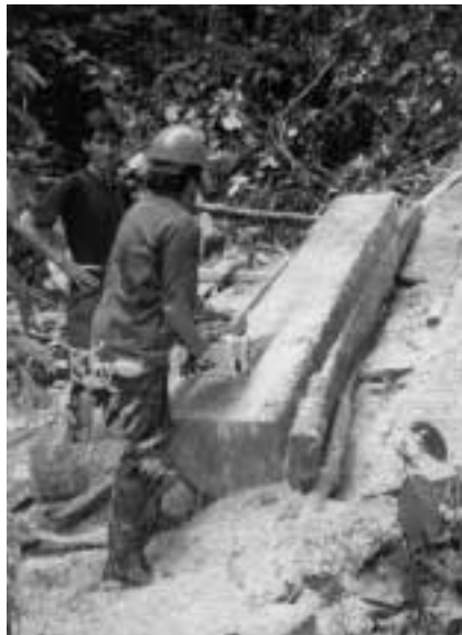
Segundo Moreno milling a hardwood tree into rough-sawn boards with a chainsaw. Such technique leaves over 50% of the usable wood wasted in the forest and greatly increases the rate of harvest for the same economic return.
